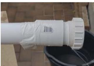
Two solvent weld inspection caps were gaffer taped to the ends of the 3mt. length of pipe to keep sand in place.
