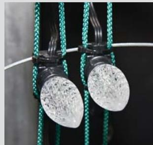
This was my original way of mounting pixels using para cord and cable ties.
