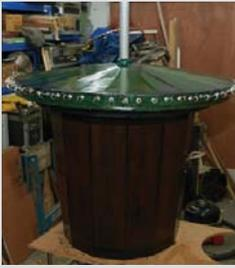
At the same time I made a new base for the tree as I had a stability problems when rigging due to a narrow base of the previous design. I also added a winch (now motorised) as the increase in lamps required this to lift the LED strings in place.
